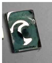
Fig. 2 This glass slide was completely even. It got a wavy surface during heat treatment.
