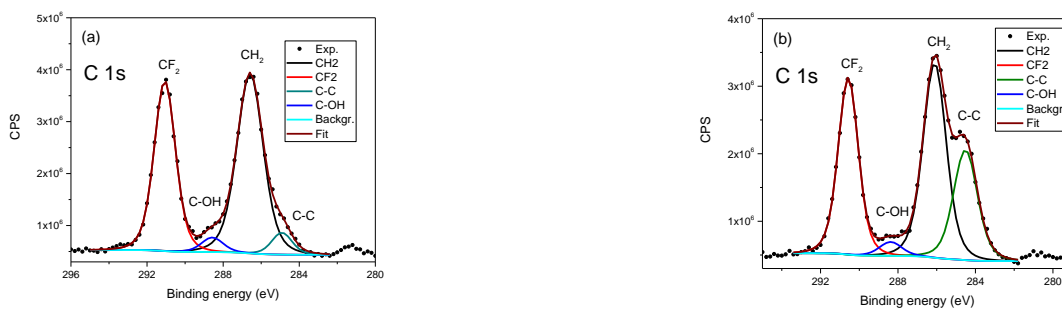
Fig. 1 C 1s orbital in unmodified PVDF polymer (a) and after 50 pulses of EUV irradiation (b).
