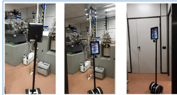
Fig. 1 A Telepresence Robot operating at TwinMic beamline.
