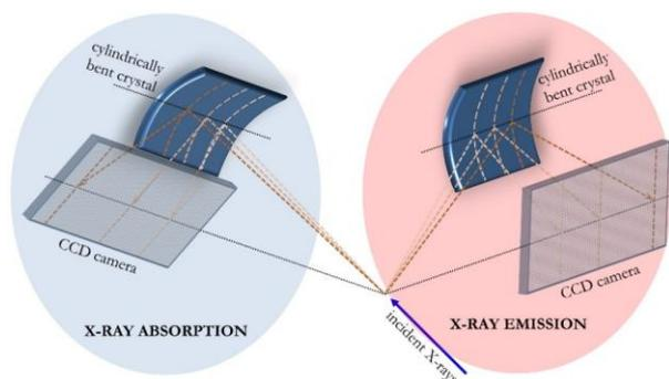
**Fig. 1.** Scheme of two von Hámos spectrometers sharing the same excitation X-ray source. In this arrangement one spectrometer measures the X-ray absorption spectrum and other measures simultaneously the X-ray emission spectrum.
