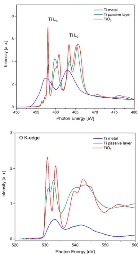
**Fig. 2.** Example of application. The Ti L-edge and O K-edge XAS spectra collected for TiO<sub>2</sub> based system (courtesy of Dr A. Wach, INP PAN, Kraków).
