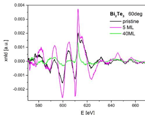
**Fig. 3.** XNLD at Te M<sub>45</sub> edge collected from pristine and Au covered Bi<sub>2</sub>Te<sub>3</sub> single crystal. The amplitude of the oscillations is a measure of anisotropy in the local structure of surface Te.
