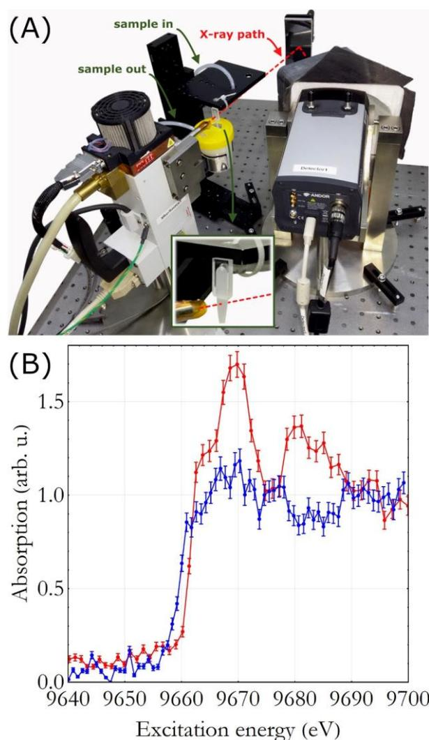
**Fig. 2.** (A) View on the experimental setup used. The X-ray tube was operated at the voltage of 30 kV and the current of 0.9 mA. (B) The Zn K-edge XAS spectra measured for the ZnO aqueous solution in the form of a jet (red) and for a Zn metal foil (blue).
