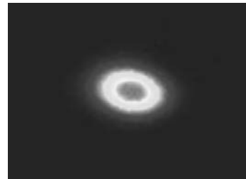
Figure 1. The image of the electron beam at 250 mA, horizontal/vertical emittances are 7.893/0.0626 nm respectively
